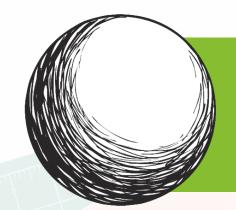
Contour-hatching follows the contour, or curve or outline, of the object. In this case, the hatching is rounded to match the shape of the circle.
